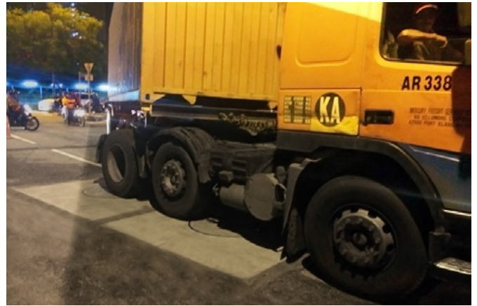
D400 load rated FL90 covers tested to EN124
